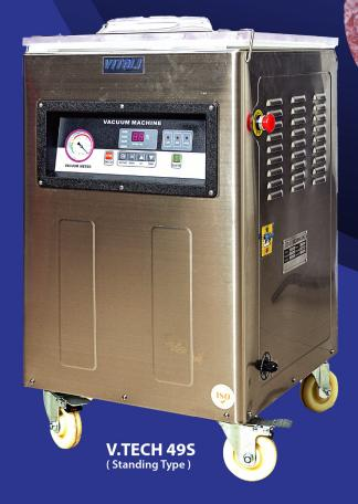
Model V.TECH 49S **Power of Motor** 1.6 kW / 1PH Voltage 220V / 50Hz **Packing Speed** 2-3 times / min **Ultimate Vacuum** 0.5 mbar **Sealing Length** 490 mm **External Dimension** 580 x 640 x 870 mm **Stock Code** 880325023
